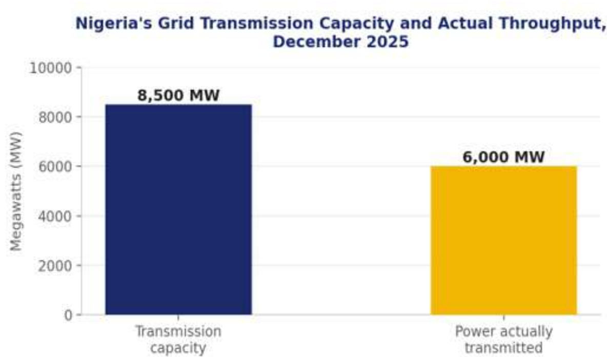
Figure 2: Nigeria’s Grid Transmission Capacity and Actual Throughput, December 2025
